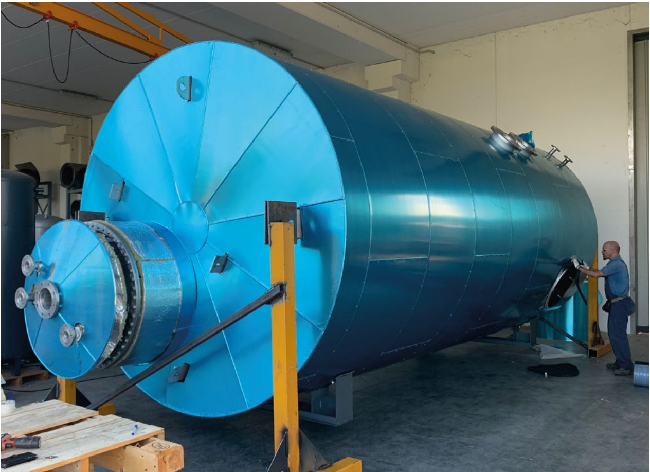
40.000 L stainless steel storage The Coca Cola Company - Netherlands
